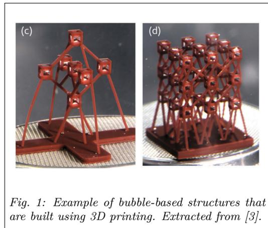
*Fig. 1: Example of bubble-based structures that are built using 3D printing. Extracted from [3].*
