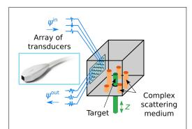
Fig. 1: Principle of the acoustic experiment that will be developed in order to maximize the amount of information enclosed in measured waves regarding the properties of a hidden target, such as its position z.
